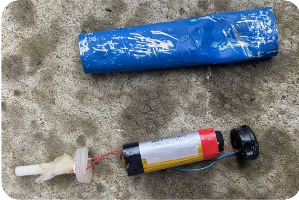
Figure 15. Basic teardowns of two widely consumed SU-ecigs
