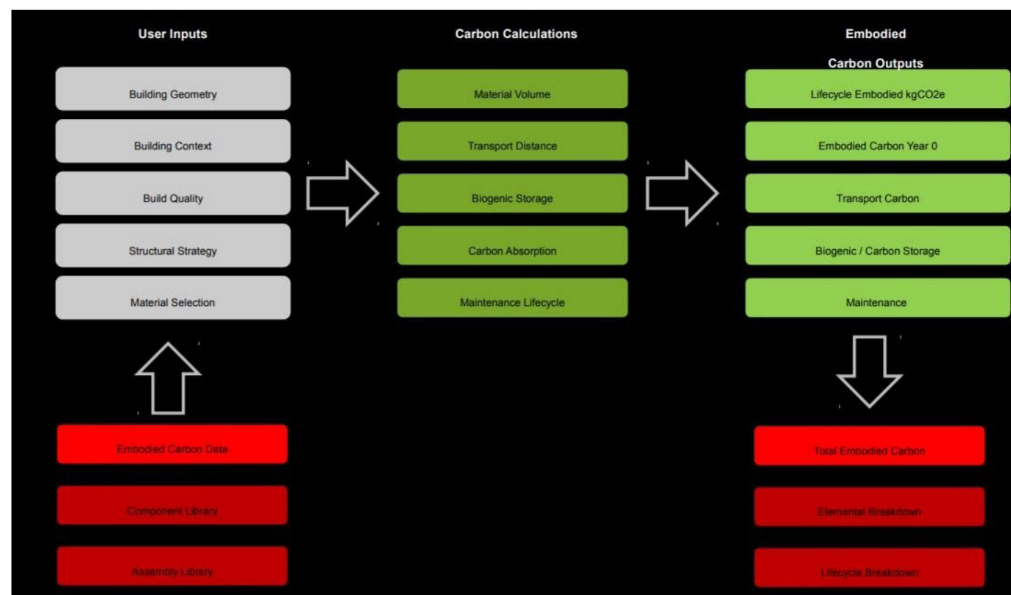
Figure 9: Workflow of the ECCOLAB tool for whole life carbon assessment. Source: (Rapiere, 2019)
