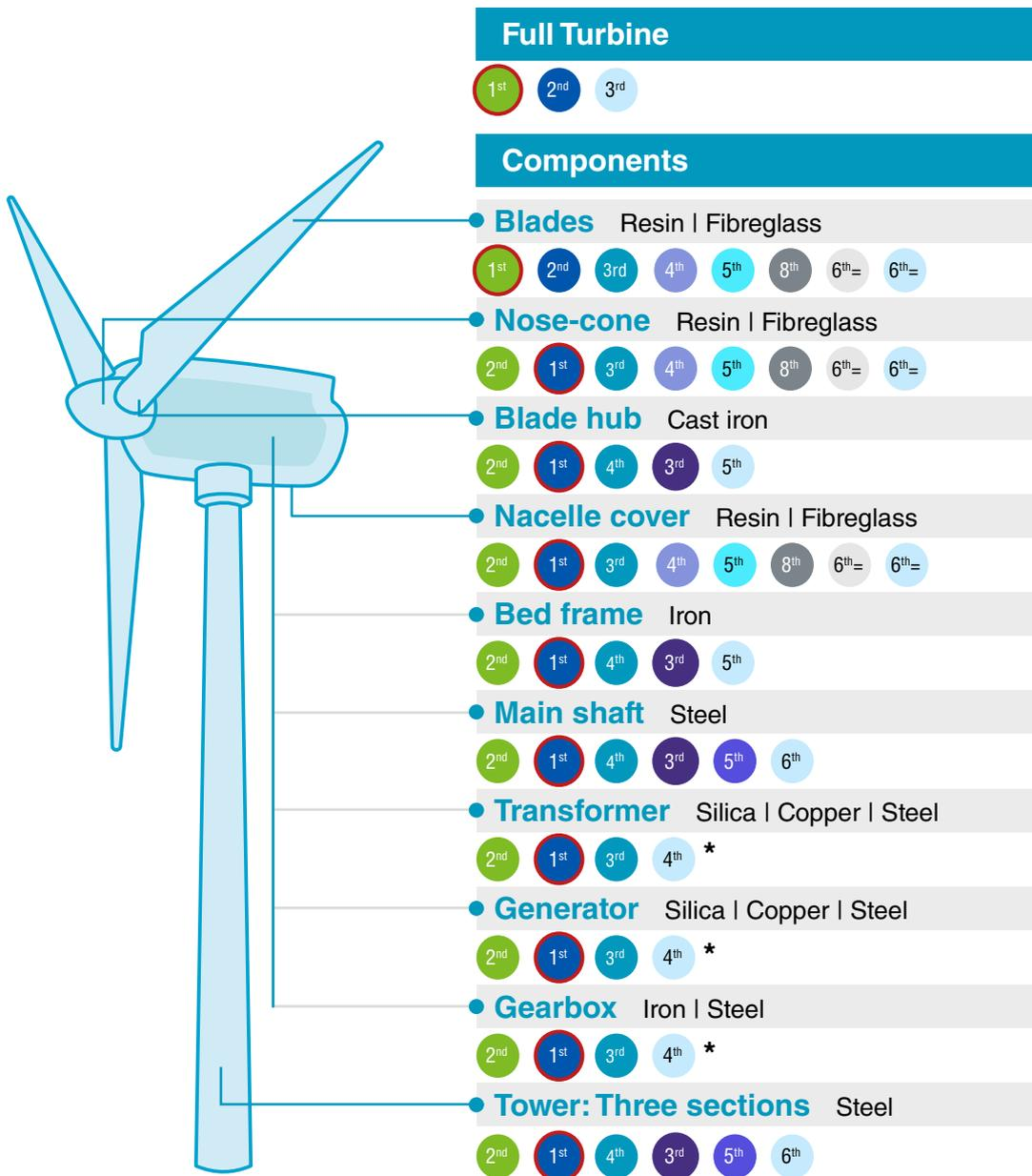
*\*Transformers generators and gearboxes consist of multiple components and materials that cannot be processed as one, therefore recycling options are not addressed in the infographic. The treatment methods for materials within these components are addressed in Table 3.4.*
