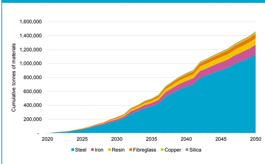
Around 80% of a wind turbine is currently recyclable; however, the biggest size categories of turbine may still require ~100 tonnes of material to be landfilled, per asset. Furthermore, there is extremely limited data available to confirm actual disposal or recycling destinations of materials from decommissioned assets.
