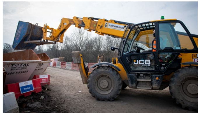
Figure 2: Tele-handler filling a timber skip
