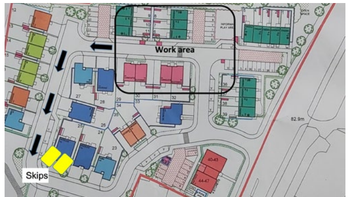
Figure 3: Site layout drawing marked up with route of tele-handler
