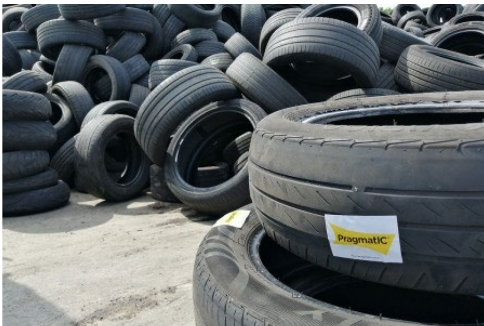
Figure 6-2 RFID tags fitted to tyres as part of a UKRI-funded waste tyre tracking project 123
