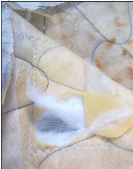
Figure 2.1 Example of the multiple layers and materials present in mattress ticking
