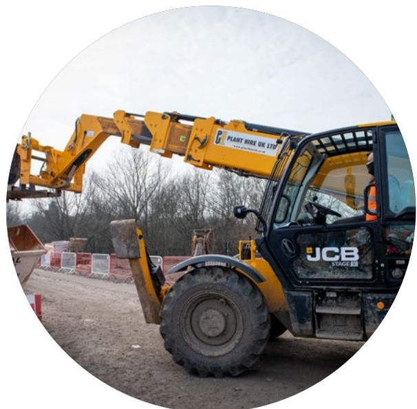
Figure 1: telescopic forklift at skip
