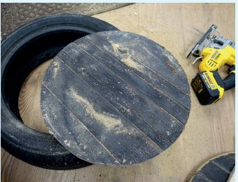
For the centre of the round, choose a spot from where you can draw a circle that includes the widest possible piece of wood on both sides. If you are left with a small strip of wood on one side of the circle, it will be difficult to make it hold together with the other pieces.
