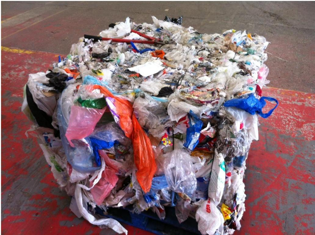
The target feedstock considered for this report is low-grade film that is too highly contaminated or otherwise unsuitable for reprocessing and recycling. There are two major sources of this type of material, namely MRFs sorting and processing municipal waste and composting facilities, although other potential sources include process residues from anaerobic digestion facilities.
